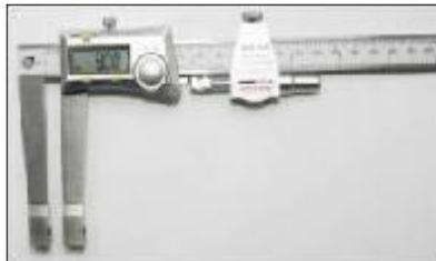
Holder assembly is not necessary when caliper YTMT203 is used
