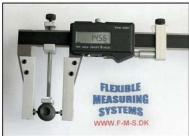
Caliper with holders 10A, pressure device 40A & centre-stop 55A measuring a M16x2-6g screw thread.
