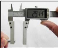
4. Remove the alignment cylinder.
