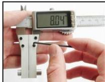
3. Fasten the four (4) grub screws carefully.
