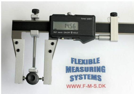
External pitch diameter measurement with holders 10A, pressure device 40A, centerstop 55A and external thread pitch diameter measurement inserts.
